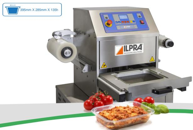
FoodPack 400 is a compact traysealer which is ideal for small and medium-sized companies. The model, which can also perform skin packaging, is able to thermoseal about 400 cycles/hour. The sealing area is 400×290 mm and it is possible to use moulds of up to 2 cavities, thus doubling productivity.
