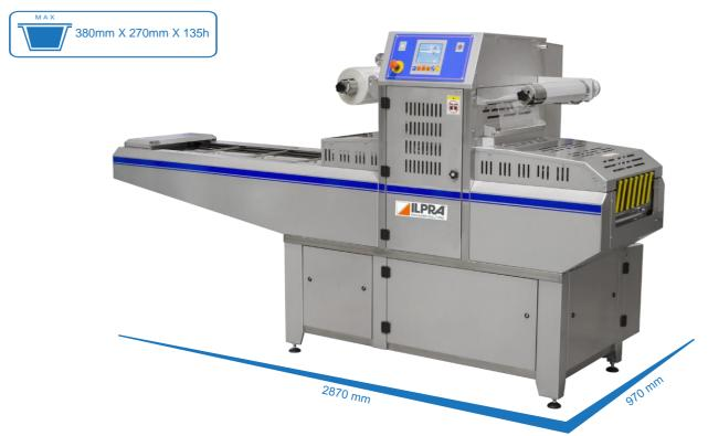
FoodPack Speedy is a compact traysealer which is ideal for small and medium productions. The machine, equipped with a touch screen monitor, is easy to use and manage because its internal components can be easily accessed. The proportional electronic film unwinder, the drawer-like mould changing and Ilpra ProGas technology ensure high performance and low consumption. The work area is 380 x 270 mm.
