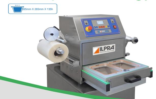
The compact, stainless steel FoodPack Energy model has a work area of 395 x 265 mm and a high sealing capacity. The motor driven film unwinder and quick changing of the mould make it flexible and fast to use for small/medium productions. Ilpra Progas technology increases its performance and reduces consumption.
