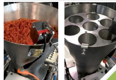
DOSING SYSTEM FOR SOLID - GRANULAR PARTICLES
