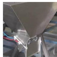
Discharge chute + timing hopper
