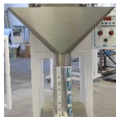
Additional discharge chute
