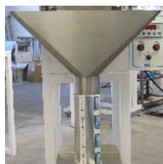
Additional discharge chute
