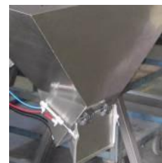
Discharge chute + timing hopper
