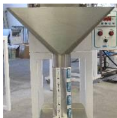
Additional discharge chute
