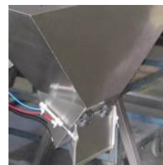
Discharge chute + timing hopper
