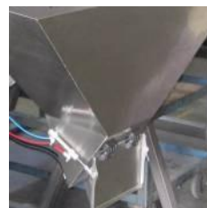
Discharge chute + timing hopper
